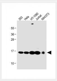
All lanes: Anti-Mouse) Rbx1 Antibody (C-term) at 1:1000 dilution Lane 1: 293 whole cell lysate Lane 2: Hela whole cell lysate Lane 3: HT-1080 whole cell lysate Lane 4: Jurkat whole cell lysate Lane 5: NIH/3T3 whole cell lysate Lysates/proteins at 20 µg per lane. Secondary Goat Anti-Rabbit IgG, (H+L), Peroxidase conjugated at 1/10000 dilution. Predicted band size: 12 kDa Blocking/Dilution buffer: 5% NFDM/TBST.
